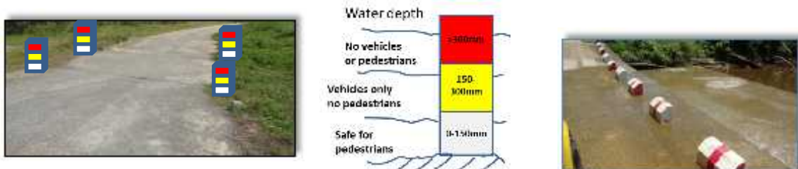
Figure 63 - Thresholds for Vehicle and People Stability in Floods
