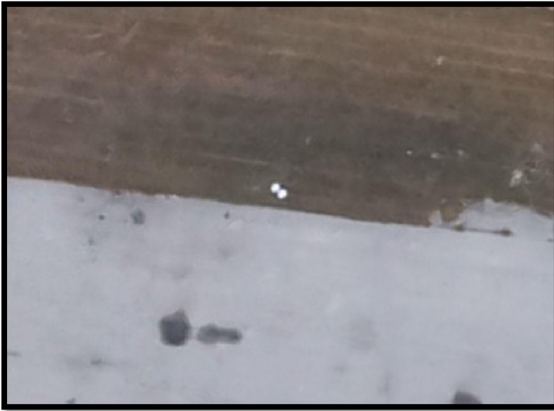
Figure 15. Ground marker seen in the centre of the image deployed on a ground control point, captured by the UAS flying at 315 m Height above Ground.
