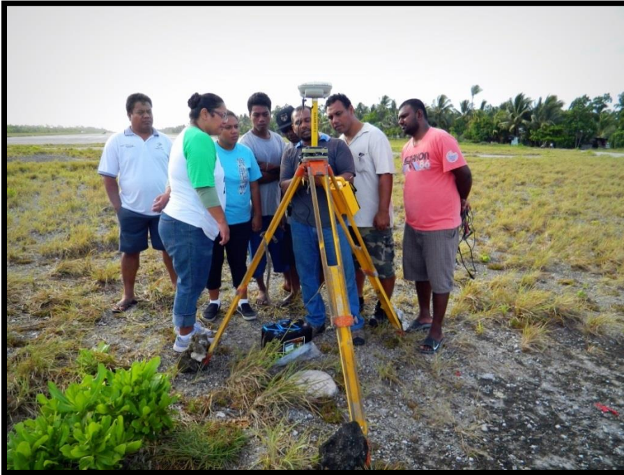
Figure 7. Setting up the base station at the BON4 benchmark.
