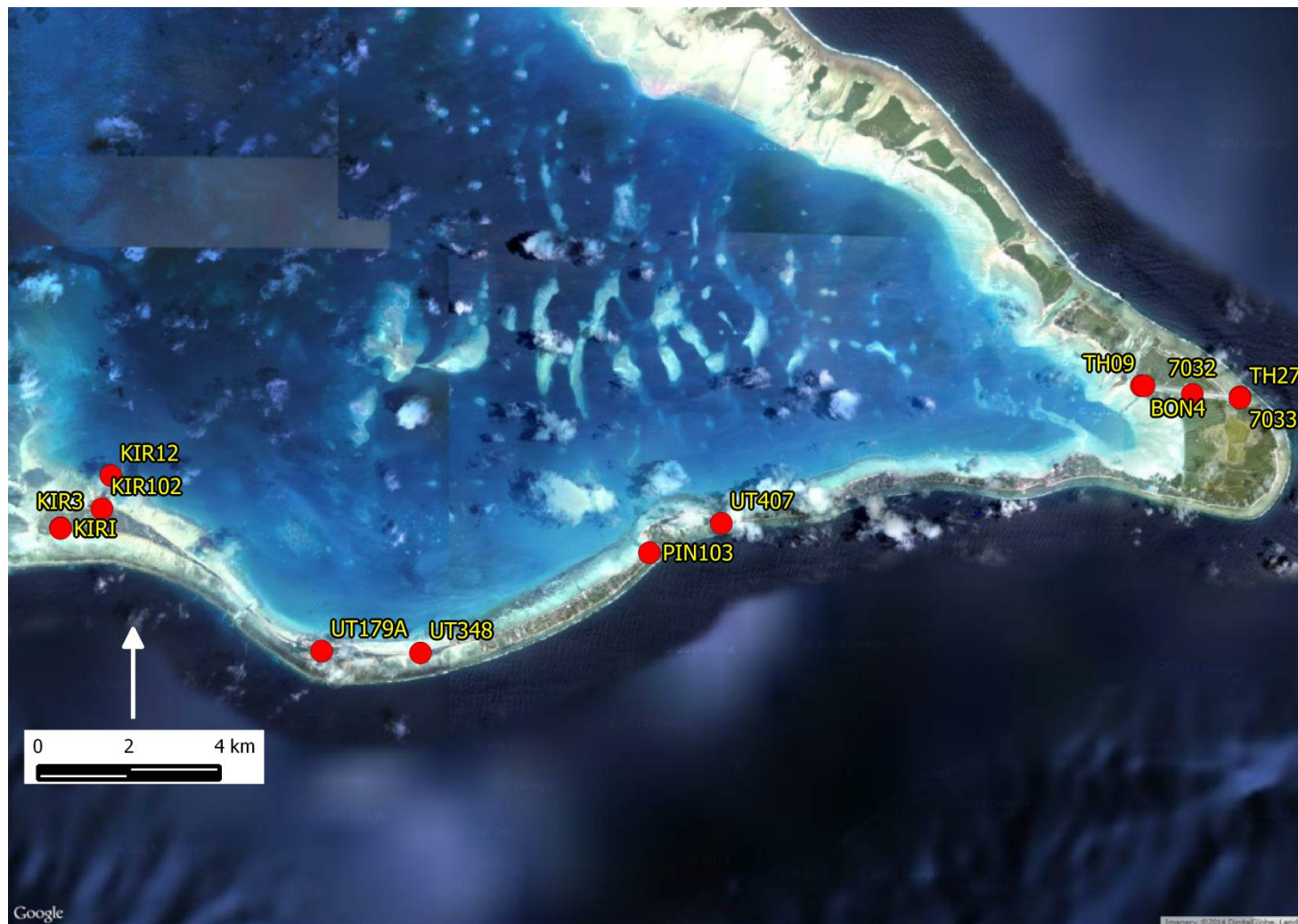
Figure 4. Locations of surveyed benchmarks for the datum investigation plotted on a Google satellite backdrop.
