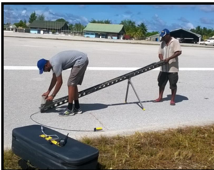
Figure 14. Trimble UX5 launching ramp used to propel the UAS into the air at high speed.
