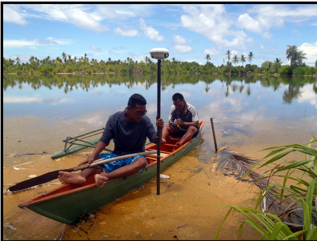
Figure 12. A canoe was used in the RTK survey in the lakes and salt water marshes.
