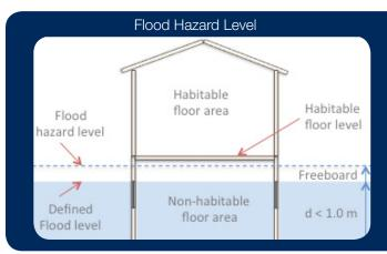
ing. Or they can be built as seals on the home itself. The idea behind these systems is to keep water outside a building while having the habitable floor level below the expected flood height.
