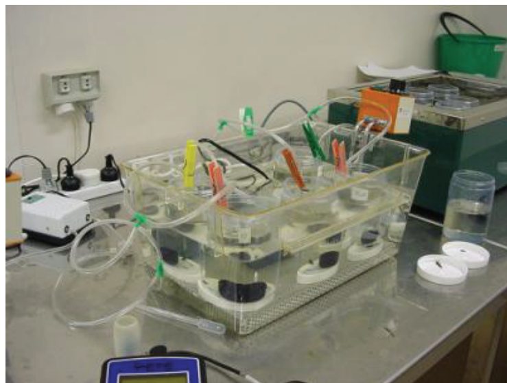
Figure 2. Experimental set-up for determination of LT 50 , showing replicate experimental units in constant temperature water bath.
